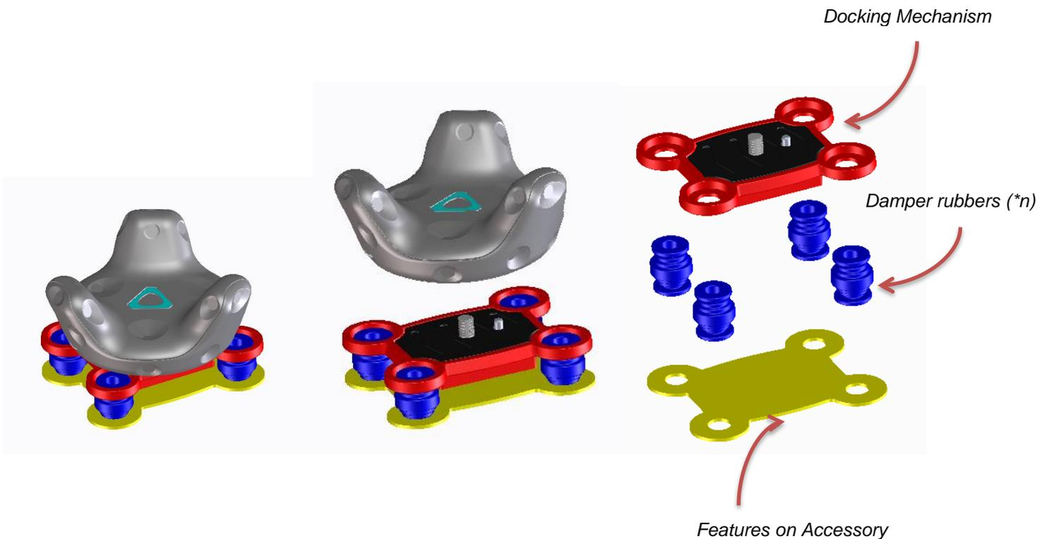
When considering the vibration level that the VR content plans to adopt, among the factors that can be adjusted are the durometer of the damper rubber, the mounting distance/position, and the usage of damper rubbers.
